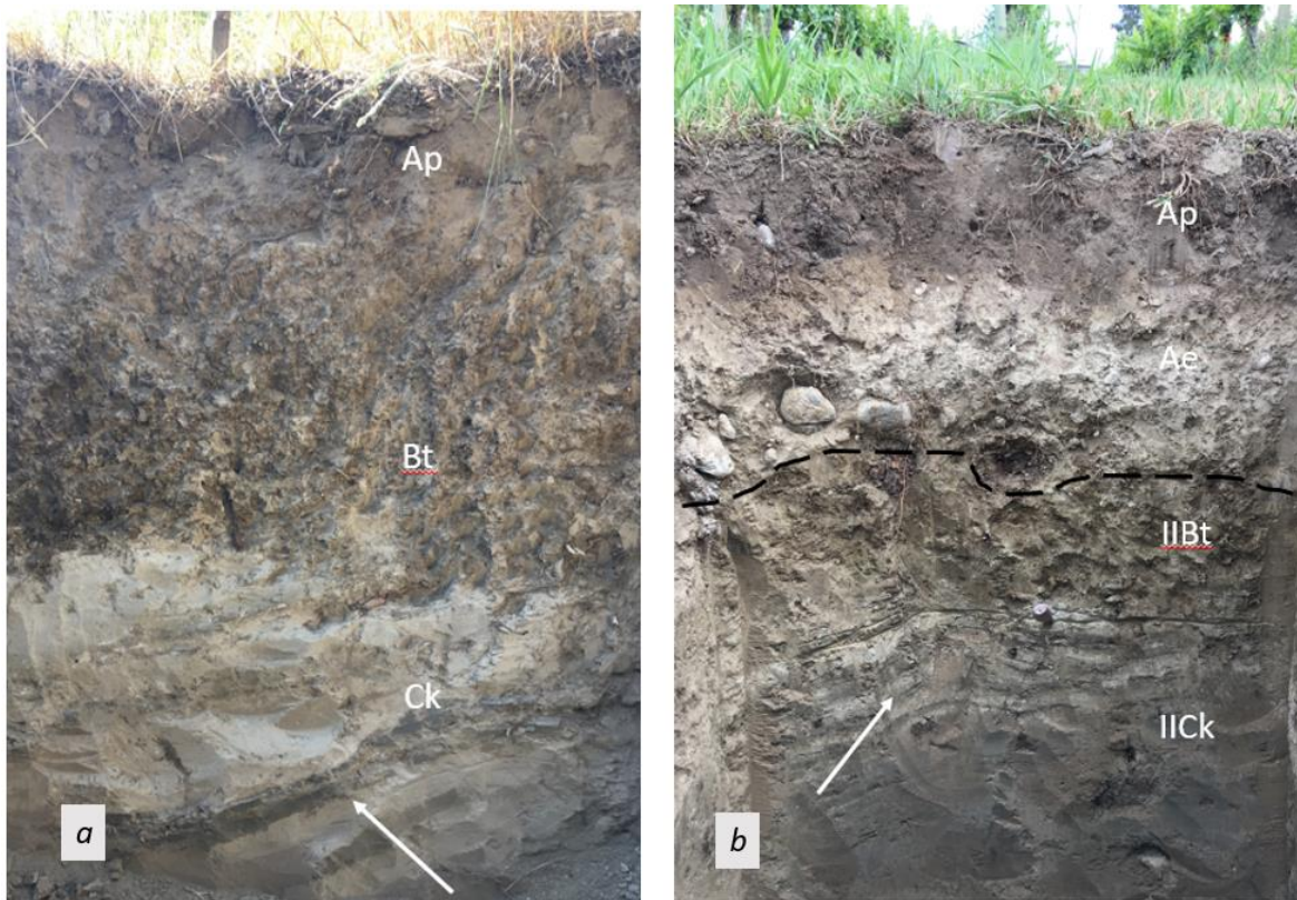
Figure 7. Soils formed in glaciolacustrine materials. When the entire soil is formed within these fine-textured materials they are classed as Boucherie soil series (a). When the glaciolacustrine materials are buried by gravelly sediments they are classed as Greata soil series (b). The lettering on the soil profiles refer to the type of soil horizon, leached layers are designated as Ae horizons, layers with accumulated clay are designated as Bt horizons, surface cultivated horizons as Ap horizons and the unweather glaciolacustrine parent material seen at the base of each profile as Ck horizons. The white arrows point to the sedimentation layering (referred to as varves) within the parent materials indicative of annual variations in glacial lake sedimentation.
