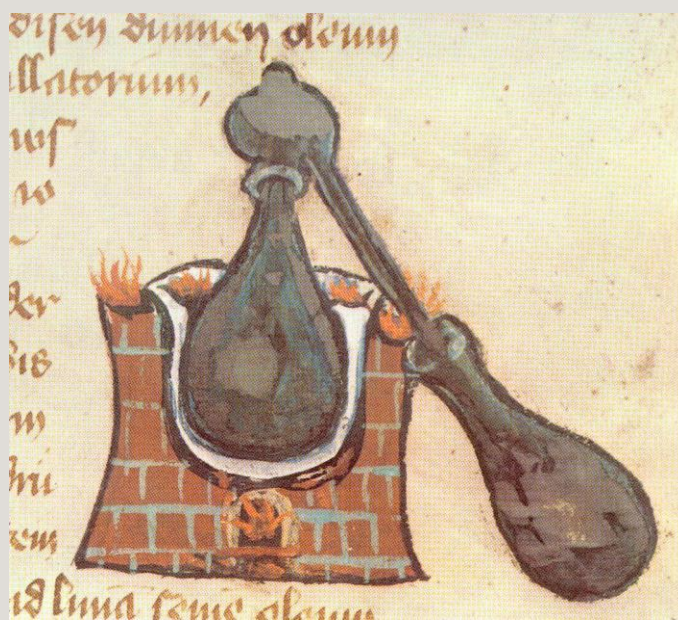
Medieval drawing of a still Three components: cucurbit, cap, and vessel
